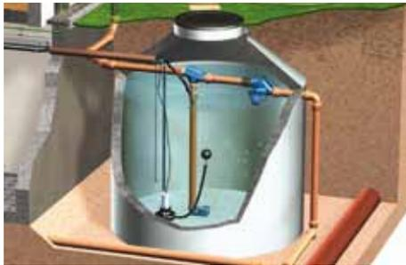
80% of the average intensity of rainfall in Germany is under 15 l/(sxha), resulting a volume flow rate of 0,32 l/s with a roof area of 213 m<sup>2</sup>.
